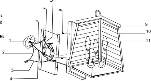
For OUTDOOR USE fixture, After completing installation, caulk fixture mounting surface with silicone weather sealant(Not Included)
