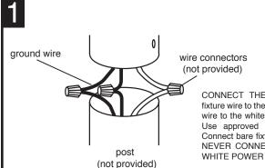
CONNECT THE WIRES. NOTE: Attach the black fixture wire to the black supply wire, the white fixture wire to the white supply wire. Do not mix them up. Use approved wire connectors (not provided). Connect bare fixture ground wire to supply ground. NEVER CONNECT GROUND WIRE TO BLACK OR WHITE POWER SUPPLY WIRES.
