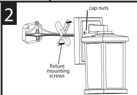
POSITION THE FIXTURE HOUSING over the fixture mounting screws and secure in place with the cap nuts provided.
