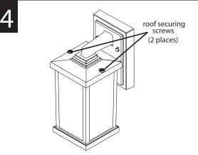
To remove cage from roof, loosen the two roof securing screws
