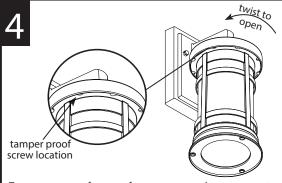
NOTE: FIXTURES IS PROVDED WITH A TAMPER PROOF SCREW TO PREVENT REMOVAL OF CAGE.
