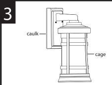
SCREW BULB into socket. Be sure to use bulb with wattage no greater than specified on fixture. NOTE: Cage does not have to be removed to install bulb.
