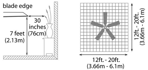
This fan can be mounted with a **downrod** on a regular (no-slope) or vaulted ceiling. The hanging length can be extended by purchasing a longer downrod (0.5in./1.27cm diameter). Other installation, such as **flushmount**, is *not* available for this fan.
