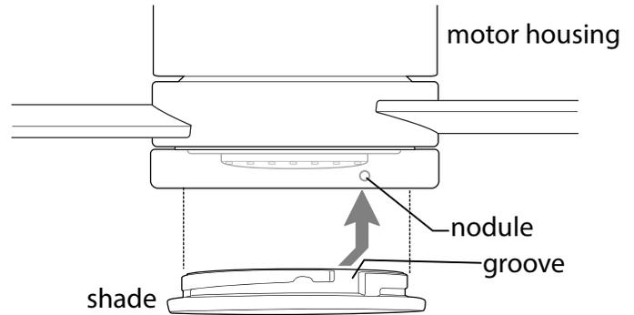
**If you do NOT wish to use the light**, locate grooves on metal cover and align with nodules inside fitter plate. Gently push up on metal cover and turn to the RIGHT (clockwise) until it no longer turns.
