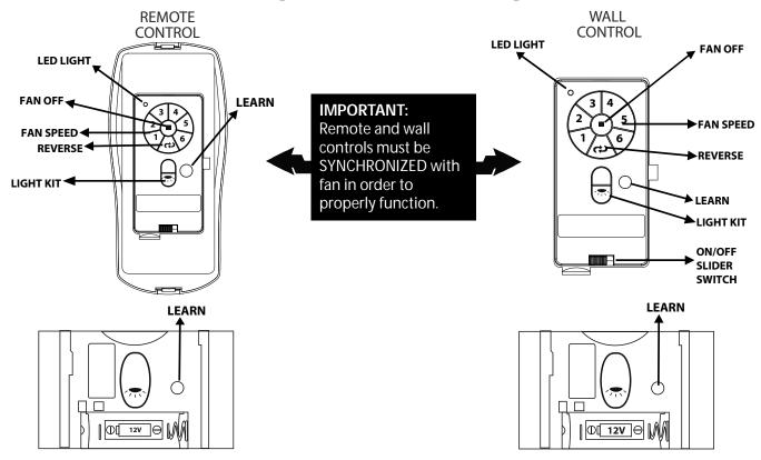
Install battery (provided) in transmitter and wall control (if applicable). **WARNING**: Battery is to be inserted with the correct polarity.
