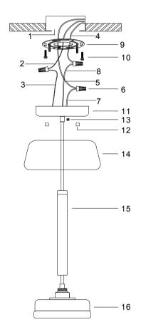
1.OUTLET BOX(not included) 2.SUPPLY GROUND WIRE(not included) 3.FIXTURE GROUND WIRE 4.BLACK SUPPLY WIRE(not included) 5.WHITE SUPPLY WIRE(not included) 6.WIRE CONNECTORS 7.RIBBED(or WHITE) FIXTURE LEAD WIRE 8.SMOOTH(or BLACK) FIXTURE LEAD WIRE 9.MOUNTING PLATE 10.OUTLET BOX SCREWS(pre-attached) 11.CANOPY 12.DECORATIVE NUT 13.SCREWS 14.OUTER GLASS SHADE 15.ROD 16.FIXTURE
